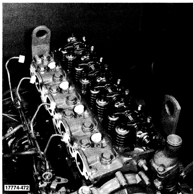
Exhaust Manifold Removed
