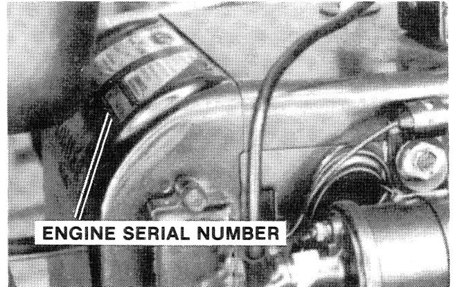
Figure 3 (10, 12, 14 & 16 H.P.) Location of Engine Serial Number
