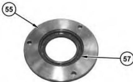
4. Apply Tooling (E) to the outer diameter of lip seal (57). Use Tooling (C) and a suitable press to install lip seal (57) into retainer (55). Install lip seal (57)
