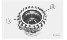
10. Remove Duo-Cone seal (12) from adjusting nut (11).
