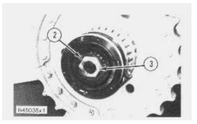
**3.** Remove lock (2) and nut (3) from the sprocket shaft.
