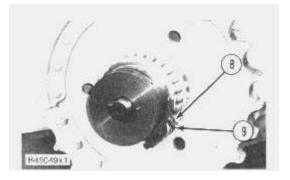
7. Remove the nut and bolt (8). Remove lock (9) from the holder assembly.
