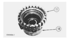
12. Remove adjusting nut (11) from holder assembly (10).
