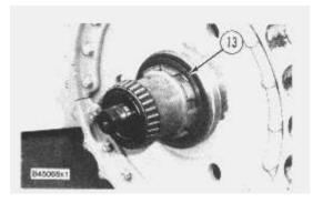
**11.** Remove Duo-Cone seal (13) from the sprocket.
