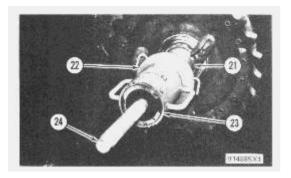
**b)** Install 5P5207 Stud (22) in 5P6222 Adapter (21). Slide 5P5212 Plate Assemly (22) and 5P5201 Cylinder (23) with the piston end away from the sprocket over stud (24) and against adapter (21).
