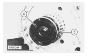
4. Remove retainer (4) and the shims from the sprocket shaft.
