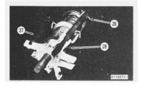
**d)** Put 6V3125 Arms (27) in position in the head and the adapters and install 6V3126 Pins (26) and 6V3127 Locks (28).
