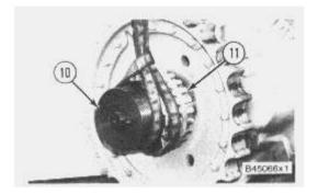
**9.** Remove tooling (A). Fasten a hoist and remove holder assembly (10) and adjusting nut (11) as a unit. The weight is approximately 80 lb. (36 kg.).
