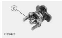
16. Remove guide (32), the two races and bearing from the sleeve.
