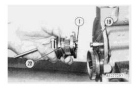
**6.** Install the weight assembly on the fuel injection pump housing with piston (1) engaged over the groove in rack (19). Install lock (20) and the bolts that hold the weight assembly to the fuel injection pump housing.
