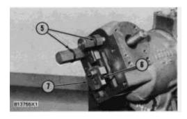
4. Remove O-ring seals (5) from the low and high idle adjustment screws.
