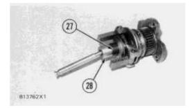
14. Remove ring (27) and the dowel under the ring that holds seat (28) in place.
