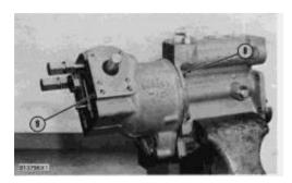
6. Remove bolts (8), and remove governor housing (9) from the fuel injection pump housing.
