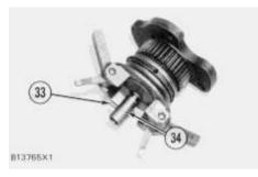
17. Remove the second dowel (33) that holds sleeve (34) in place, and remove the sleeve.
