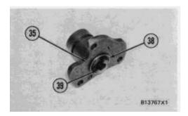
20. Remove sleeve (38) and piston (39) from cylinder (35). Remove the O-ring seal from the sleeve.
