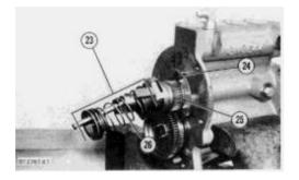
**12.** Remove seat, washer, wave-washers and governor spring (23) from the weight assembly. Remove spring washer (26) from the weight assembly.
