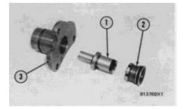
**1.** Install the O-ring seal on sleeve (2). Install piston (1) in sleeve (2). Install sleeve (2) in cylinder (3).
