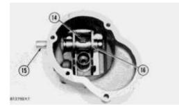
**9.** Remove bolt (14) and the lock. Remove shaft (15) and lever assembly (16) from the governor housing.
