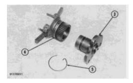
2. Install cylinder (3) in weight assembly (4), and install lock (5) to hold them together.
