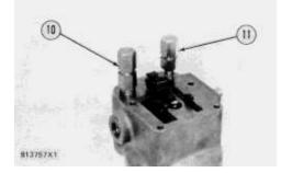
7. Remove high idle adjustment screw (11) and low idle adjustment screw (10) from the governor housing. Remove the high idle adjustment screw first.
