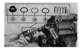
7. Install spring washer (26) on the bolt as shown.
