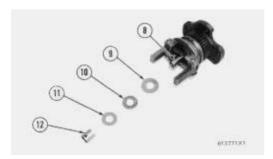
**4.** Install larger race (9), bearing (10), smaller race (11) and guide (12) on sleeve (8). Put the hole in guide (12) in alignment with the first hole in sleeve (8).
