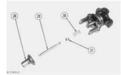
**15.** Remove seat (28), bolt (29) and spring (30) from the weight assembly. Remove washer (31) from spring (30).
