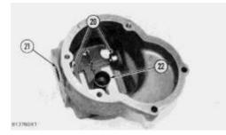
**11.** Remove seal (21) from the governor housing. Use tooling (A) to remove the plug and bearings (20) from the governor housing.
