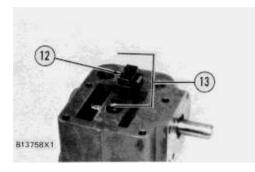
8. Remove bolts (12) and torque control (13) from the governor housing.
