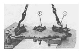
**7.** Install tooling (C) and fasten a hoist as shown. Remove the bolts that hold the cover to the housing. Remove cover (8). The weight is 80 lb. (36 kg).
