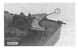
6. Remove alternator bracket (7) from the pump drive.
