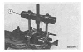
**4.** Install tooling (B) as shown. Use tooling (B) to loosen the pulley from the taper. Remove tooling (B), nut (4), washer (5) and pulley (6). Remove the key from the gear.
