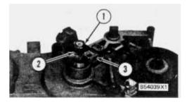
**1.** Loosen nut (1) until washer (2) is approximately-1/8 in. (3.2 mm) away from yoke (3). Do not remove the nut at this time.
