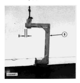
**5.** Adjust the lifting shackle on tooling (B) so distance (X) is **38 mm (1.5 in).** The lower mounting bracket should be installed so the spacers are out as shown.
