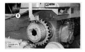
**6.** Remove two bolts from the sprocket segments. Fasten a hoist, and install tooling (B) on the final drive as shown.
