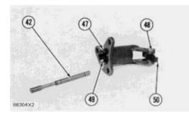
**23.** Remove valve (42), sleeve (47) and piston (49) from the governor servo. Remove the O-ring seal from sleeve (47).
