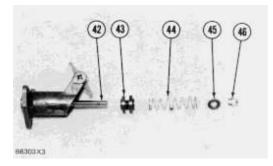
**22.** Remove lockring (46), seat (45), spring (broken link spring) (44) and sleeve (43) from valve (42). Remove the other lockring (46) from the groove in the center of valve (42).
