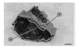
11. Remove shaft (22) and lever (23) from the housing.
