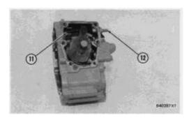
7. Remove low idle adjustment screw (12) and spring (11) from the housing.
