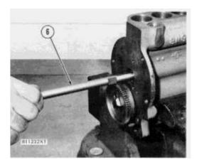
**7.** Install rack (6) in the pump housing with the groove near the end of the rack toward the governor end of the pump housing.
