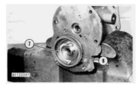
5. Remove spring (7) and gear (8) from the camshaft.
