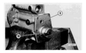
6. Remove camshaft (10) from the pump housing.
