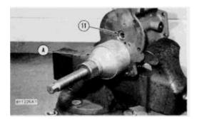
7. Remove bearings (9) and (11) from the pump housing.
