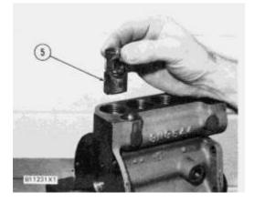
**6.** Install lifters (5) and the spacers in their original position in the pump housing. Install the lifters with the pin in the lifter on the same side as the pin in the pump housing.
