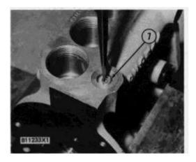
**8.** Be sure the hole in plate (orifice) (7) is open, and install plate (7) in the pump housing. Install the elbow over the plate.
