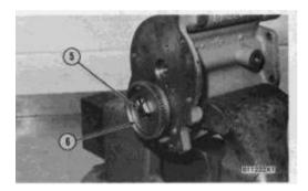
4. Remove bolt (5), the lock and plate (6) from the camshaft.
