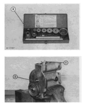
**1.** Remove elbow (1) and the plate (orifice) under the elbow.
