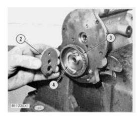
**5.** Put gear (3), spring (4) and plate (2) in position on the camshaft as shown. Install the lock and bolt that hold plate (2) in place.
