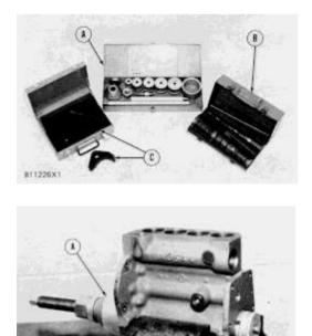
1. Install the camshaft bearings in the fuel injection pump housing with tooling (A). Install the bearing in the governor end of the housing so the lubrication hole in the bearing is in alignment with the lubrication hole in the housing. Install the camshaft bearings so they are  $0.25 \pm 0.13$  mm  $(.010 \pm .005 \text{ in.})$  below the ends of the pump housing.
