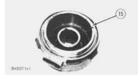
**15.** Remove cage (15) from the holder with tooling (F) as shown.
