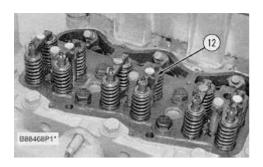
7. Put identification marks on the bridges as to their location in the engine. Remove bridges (12) from the dowels on the cylinder head assembly.
