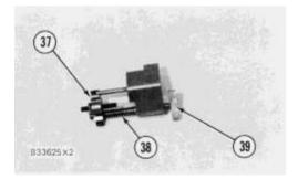
**19.** Remove the bolt that holds collar (37) to bolt (39). Remove collar (37) and spring (38) from bolt (39). Remove bolt (39) from the block.
