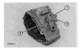
**4.** Make a mark of the position of lever (7) on shaft (8). Loosen bolt (10). Use a chisel or screwdriver to expand expansion of lever (7) so it can be removed from shaft (8).
