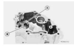
18. Remove bolts (36) and block (35) for the full load stop from the housing.
