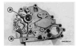
14. Remove seal (29) and adjustment screw (30) for high idle.
