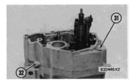
15. Remove two bolts (31), housing (32) and the gasket from the fuel injection pump housing.
