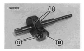
**9.** Remove two snap rings from pins (17), and remove pins (17). Remove plates (16) and stop (18) from the shaft assembly.
