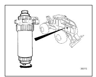
Check the glass sediment bowl of the primary fuel filter / water separator for water or debris.
