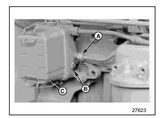
Drain and remove fuel filter (C).
