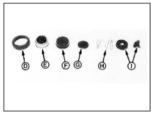
Remove hand primer from fuel filter base. Disassemble hand primer assembly (D - I) and clean.
