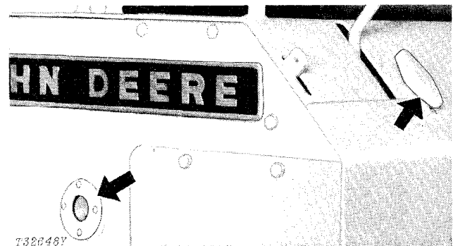
Fig. 8-Oil Level Window and Latch
