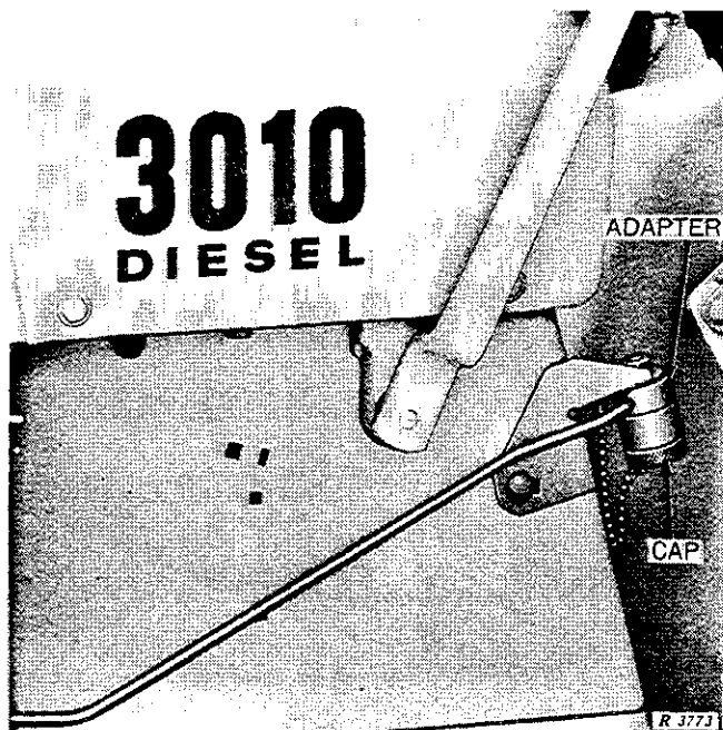
Fig. 10-10-3—Cold Weather Starting Fluid Adapter
