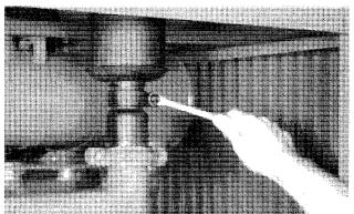
8. Remove four nuts (A) from underside of stationary hood.
