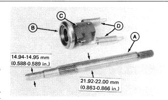
A—Drive Shaft B—Release Bearing
