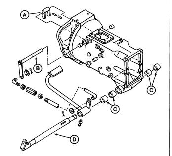
A—Clutch Yoke B—Yoke Armshaft C—Pedal Bushing D—Pedal Shaft
