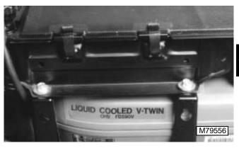
The engine serial number is located on the right side of the blower housing.
