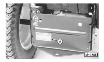
The product identification number (A) is located on the left rear corner of the tractor frame.
