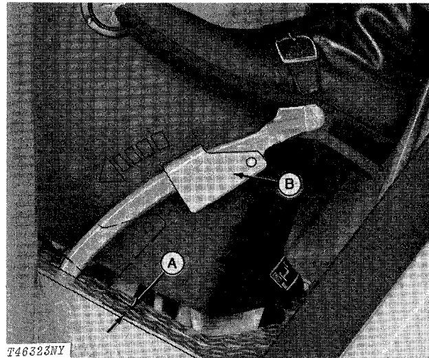
A—0.75 in. (19 mm) Maximum Clearance B—Clutch Pedal Stop
