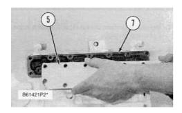
1. Install gasket (7) and cover (5) on the side of the fuel pump housing.
