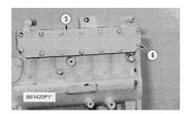
**6.** Remove bolts (6), cover (5) and the gasket from the fuel pump housing.
