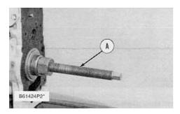
7. Use Tool (A) and install the three camshaft bearings in the fuel pump housing with the oil holes in the bearings  $30 \pm 3$  degrees from the horizontal center line toward the plugged holes in the fuel pump housing.
