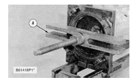
3. Use Tool (A) and remove the three camshaft bearings from the fuel pump housing.
