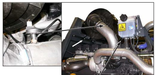
Disasssemble the cable to the Air filter sensor and cable to the sensor for the cooling water expansion tank (black arrows).
