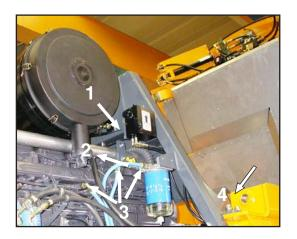
Disconnect the brake hose from the magnetic valve.
