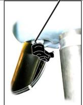
Disconnect the exhaust pipe from the turbo pipe bend.
