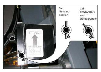
With the handle, pump and raise the cab.
