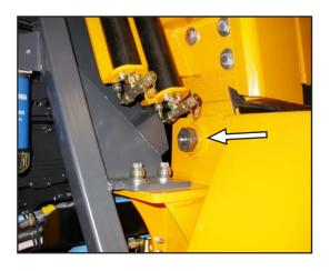
Turn the direction valve on the pump in lifting up position.
