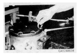
**4.** Run the eyebolts (M12) into the bolt holes from which the two bolts were removed in above step and hoist the motor using a wire rope and a crane.
