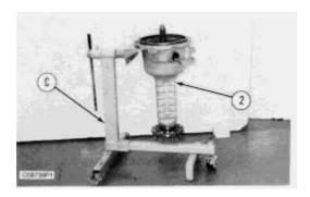
**4.** Put axle housing (2) in position on tooling (C).
