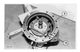
7. Remove nuts and bolts (10) to remove inner brake housing (9).
