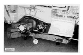
7. Lower the jack, and remove the rear axle (7). Weight of the rear axle is 450 kg (990 lb.).
