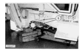
**6.** Remove four mounting nuts and bolts (6) [both sides].
