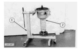
**4.** Put axle housing (2) in position on tooling (C).
