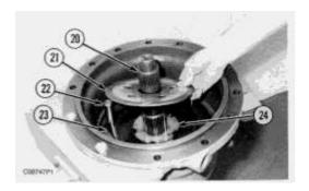
**12.** Remove sun gear (20). Remove outer disc (21), plate (23) and disc (24). Remove brake torque pin (22).
