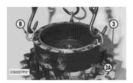
**14.** Fasten Tool (B) and a hoist to ring gear (3) as shown. Remove the ring gear from ring gear (3A). The weight of the ring gear is **23 kg (52 lb)**. Fasten Tool (B) and a hoist to ring gear (3A). Remove the ring gear from the main housing. The weight of the ring gear is **24 kg (53 lb)**.
