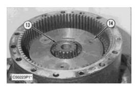
11. Remove sun gear (13) from carrier assembly (14).
