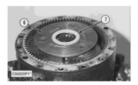
**9.** Remove spacer (7) from carrier assembly (6). Remove carrier assembly (6) by lifting it straight up.
