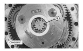
**8.** Remove sun gear (5) from the carrier assembly.
