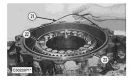
15. Remove O-ring seal (21) from the main housing.
