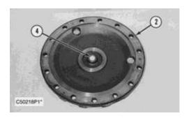
7. Remove thrust plate (4) from cover (2).
