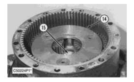
12. Remove carrier assembly (14). Remove spacer (15) from the carrier assembly.
