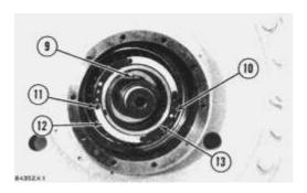
6. Remove key (9) from the shaft. Remove bolts (11), locks (12), and a lock (10).
