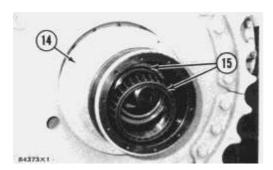
**9.** Remove two bearing cones (15) from the shaft. Fasten a hoist to the support (14) and remove it. Weight is 120 lb. (54 kg). Remove the Duo-Cone seal from the support. Remove the bearing cup from the support with a hammer and punch.
