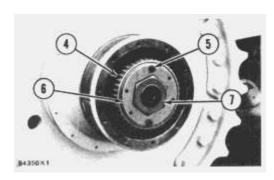
**4.** Remove bolts (5) and lock (6). Remove nut (7) from the shaft. Remove bearing cone (4) from bearing cage.
