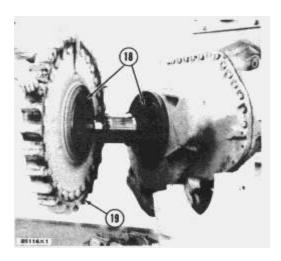
12. Fasten a hoist to the sprocket (19) and remove it. Weight is 700 lb. (318 kg).
