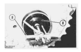
**5.** Remove bearing cage (8) with tooling (B). Remove the bearing cup from the bearing cage with a hammer and punch.
