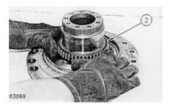
**2.** Heat bearing cone (2) to **120°** C **(248° F).**Use temperature resistant gloves to install bearing cone (2) on the spindle as shown. Make sure the bearing cone is properly seated.
