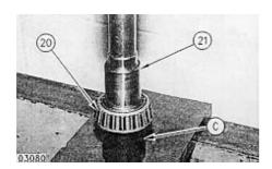
**16.** Heat bearing cone (20) to **120° C** (**248° F**). Place bearing cone (20) as shown on Tooling (C). Using a press, install shaft (21) until it is seated against Tooling (C).
