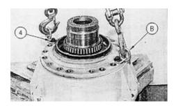
**4.** Install Tooling (B) as shown using two **M12 X 40 mm**bolts (4) and washers. Attach a suitable lifting device and position the spindle assembly on the case. The weight of the spindle assembly is **43 Kg (95 lb).**Remove Tooling (B).
