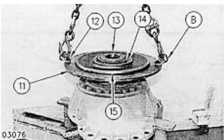
10. Install Tooling (B) on hub assembly (11) as shown using two  $1/2 \times 1-1/2$  bolts (12) and washers. Attach a suitable lifting device and position the hub assembly on spindle (13). The weight of the hub assembly is **64 Kg (140 lb)**. Remove Tooling (B) and install O-ring seal (15).
