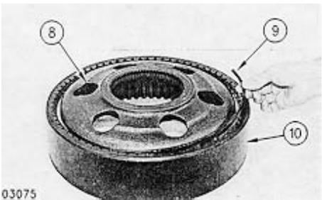
9. Install hub (8) and ring (9) in gear (10).
