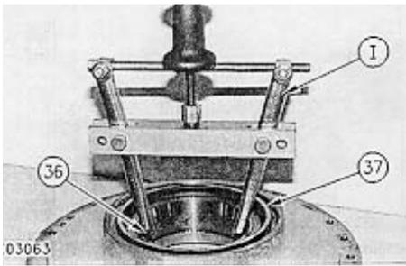
28. Using Tooling (J), remove cup (36).
