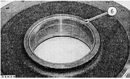
6. Lower the temperature of cup (6) and install the cup in the hub.
