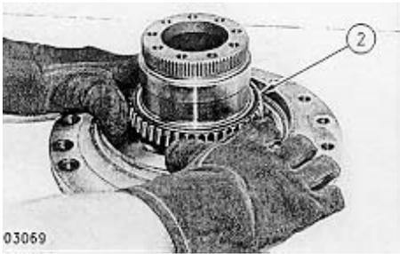
2. Heat bearing cone (2) to **120° C (248° F)**. Use temperature resistant gloves to install bearing cone (2) on the spindle as shown. Make sure the bearing cone is properly seated.
