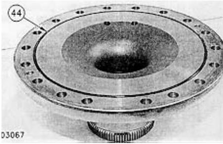
35. Turn the spindle over and remove O-ring seal (44).
