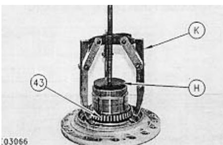
34. Using Tooling (H) and (K), remove bearing cone (34).
