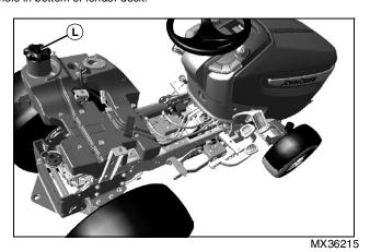
12. Immediately install fuel tank filler cap (L), being sure to not allow dirt or other debris to enter fuel tank.
