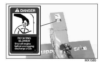
Shut off engine before unclogging discharge chute.
