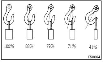
3. Do not sling a heavy load with one rope alone, but sling with two or more ropes symmetrically wound on to the load.
