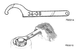
Removal and Installation of the Sprocket Wheel
