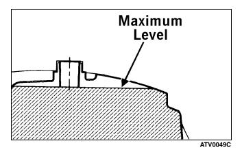
Since gasoline expands as its temperature rises, the gas tank must be filled to its rated capacity only. Expansion room must be maintained in the tank particularly if the tank is filled with cold gasoline and then moved to a warm area.
