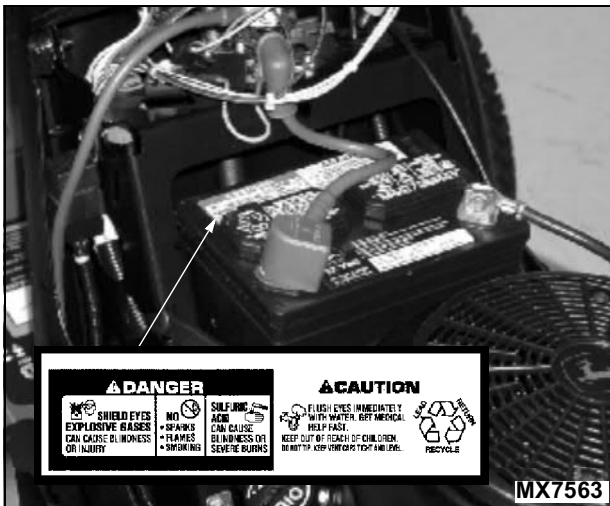
Picture Note: Located on Battery
