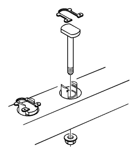
**Fig. 13: View Of Crossmember Bolt & Spring Clip - Front Courtesy of GENERAL MOTORS CORP.**
