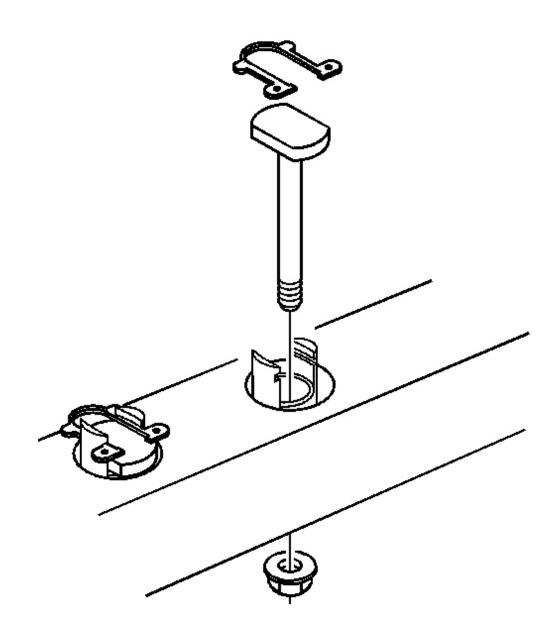
Fig. 14: View Of Crossmember Bolt & Spring Clip - Front
