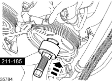
Fig. 13: Installing Pulley Using Special Tool (211-185) Courtesy of FORD MOTOR CO.
