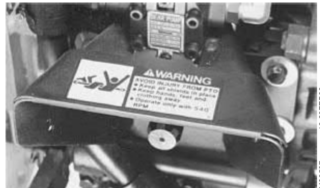
PTO Safety Sign-Rear PTO Master Shield
