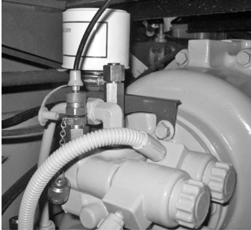
Figure 2 Test nipple with hose to gauge
