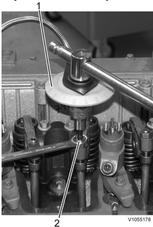
Figure 10 Grey-marked valves can be adjusted when valves for cylinder 1 overlap.
