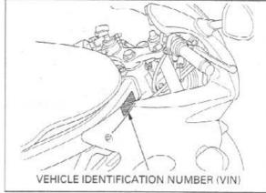
The Vehicle Identification Number (VIN) is located on right side of the frame near the steering head.
