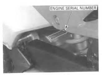
(2) The engine serial number is stamped on the lower left side of the cylinder block.
