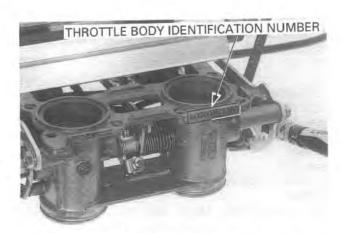
(4) The throttle body identification number is stamped on the front side of the throttle body as shown.
