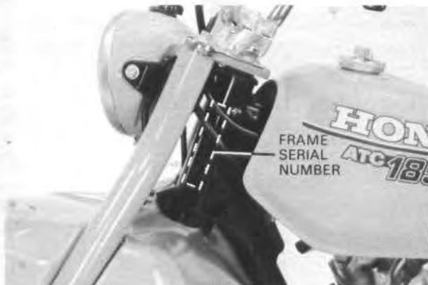
The frame serial number is stamped on the steering head left side.
