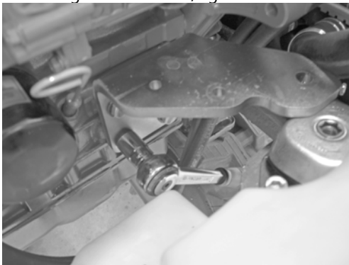
Figure 6 Engine mount, install
