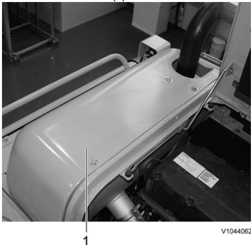
Figure 19 Installation, silencer hood
