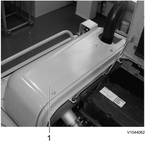
Figure 3 Removal, silencer hood
