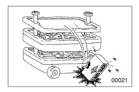
Take care when handling sensors, relays, etc. which are vulnerable to shock and heat. Do not attempt to remove the cover from, or apply paint to, the electronic control unit.
