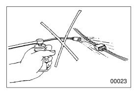
When washing the vehicle, cover the electric system parts and instruments with waterproof material beforehand (Cover with vinyl sheet or the like). Keep water away from harness wire connectors and sensors. If any of them should get wet, wipe them off immediately.
