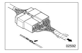
Check if harnesses are broken by pulling gently around the terminals.
