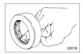
Apply the specified oil or grease to U-packings, oil seals, dust seals and bearings during assembly.
