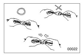
Pull the connector, and not the harness lead, to separate connectors. To separate a lock-type connector, first push toward arrow mark. To reconnect a lock-type connector, press the separated parts until they click together.
