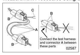
Test with connectors engaged (continuity through circuit obtained) < Waterproof connector>
