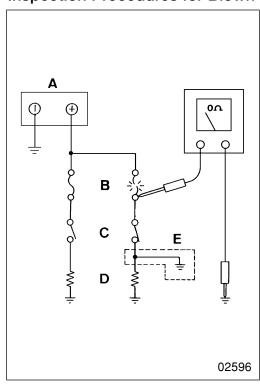
Remove fuse B and measure resistance between the loaded side of the fuse and ground.
