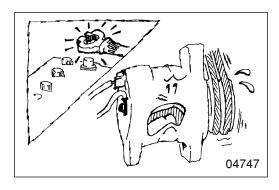
While the engine is running, do not remove the battery terminals. If the battery terminals are removed at that time, a surge voltage is generated and the diode or regulator might be weakened.
