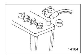
Before carrying out maintenance work on the electric system, disconnect the negative terminals of the batteries to prevent them from short-circuiting and burning-out.
