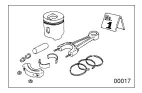
Put alignment marks on part combinations before disassembly and arrange the disassembled parts neatly. This will help avoid mismating of the parts later.
