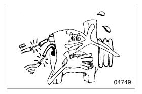
Do not short-circuit terminal B and terminal L while running the alternator.
