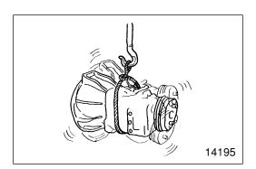
If you do not have the specified lifting hanger, secure the item using cable taking the point-of-balance of the item into consideration.
