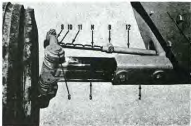
Fig. AC2 — View showing front axle extension. Toe-in should be correct for each tread width position when bolt (B) is located in proper notch (N) in tie rod. Refer to Fig. AC1 for legend.
